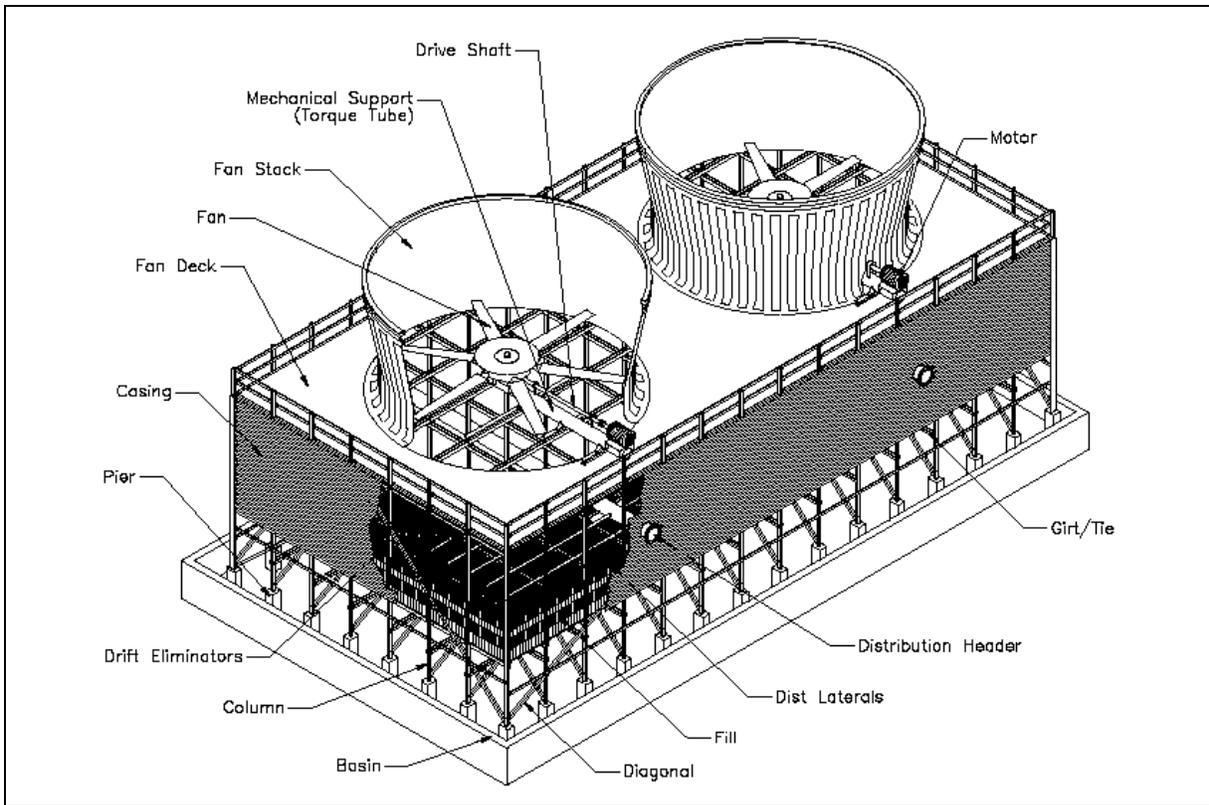
**Figure 6:** Example counter-flow cooling tower schematic
