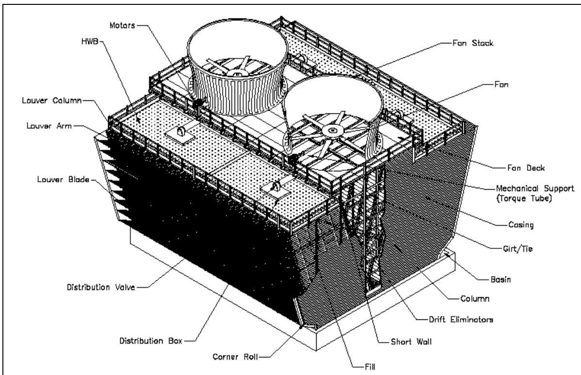
**Figure 5:** Example cross-flow cooling tower schematic
